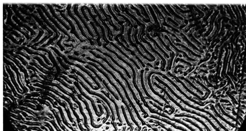
Fig. 6. The flexoelectric static domains were totally replaced by hydrodynamical ones in an MBBA layer, 26\text{ }\mu\text{m} thick, when the glasses were treated with SiO thin films followed by one layer of aliphatic monoamine \text{C}_8\text{H}_{17}\text{NH}_2 deposition on one of them. The magnitude of the applied voltage was about 3.5 V, n_0 \parallel P \parallel A . The short side of the photo corresponds to 1350\text{ }\mu\text{m} .
